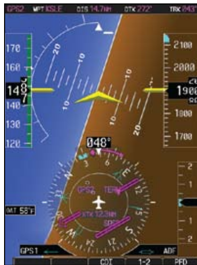
Figure 2-17 Extreme Roll Indication with Display Declutter
